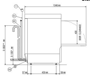
Without drain pump \*\*\*Plug only for Single Phase Machine
